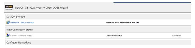
Afterward, under "Configure Networking" column, users can find networking information for each of the 2 nodes. "NICO-Cluster" stands for the heartbeat\* cable pre-installed inside CiB-9220. "NIC1-Right" stands for the networking port (the blue arrow) mentioned in page 4. Moreover, each node has a default heartbeat IP address\* (169.254.xxx.xxx) assigned by DHCP.
