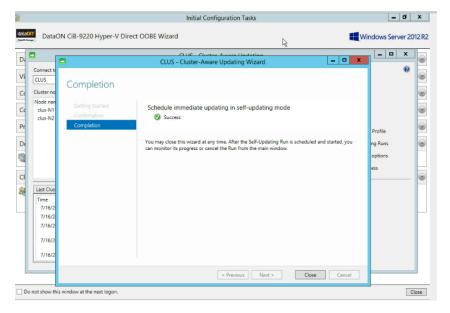
16. Shown below, the process of self-updating has started as both nodes are being updated. One node will be brought down to maintenance mode while the other node will continue to be in standby mode. Depending on complexity of the updates, estimated time for completion may vary for both nodes.
