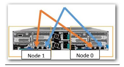
2. Prepare both nodes on screen as shown below. Please use **node 0** to configure your CiB-9220 by clicking "Yes" on the screen. Node 1 will imitate the configurations as you make on node 0 automatically from this point on. Hence, it is **NOT** necessary to switch between node 0 and node 1 in order to finish the configuration.\*
