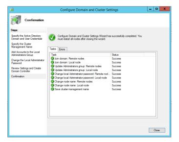
Upon completion, the wizard will ask to restart both nodes. Click "OK" to reboot (the remote node will reboot automatically; users do not need to switch between nodes to complete the restart). After restarting\*, users can begin **creating a storage pool**.
