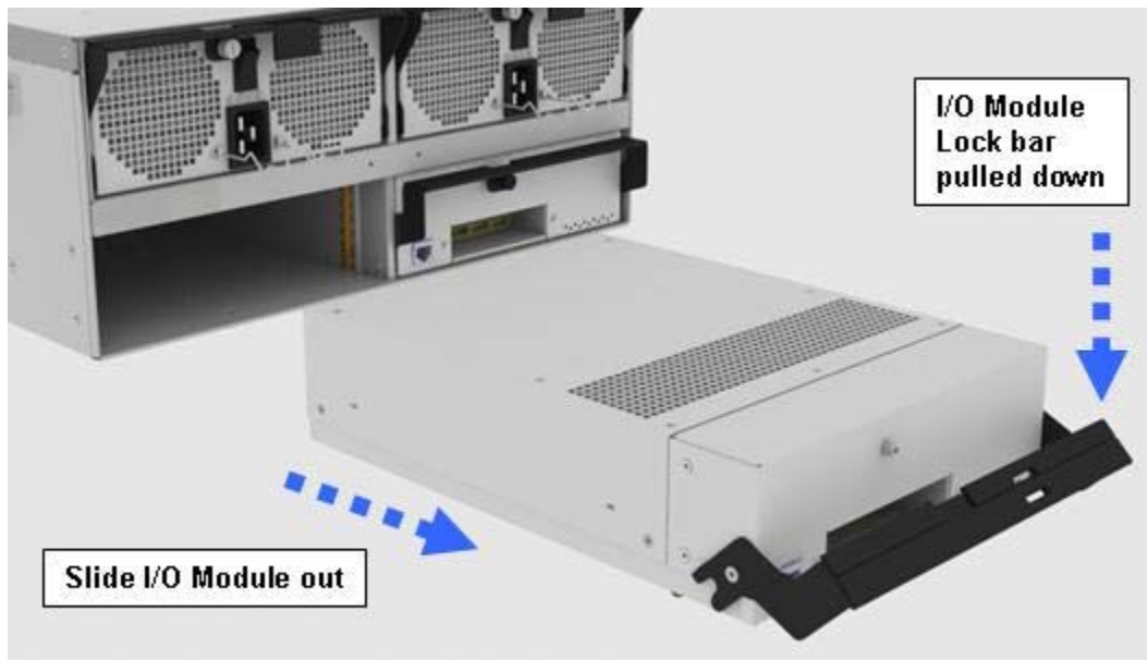
DNS-1660 I/O Module removal
