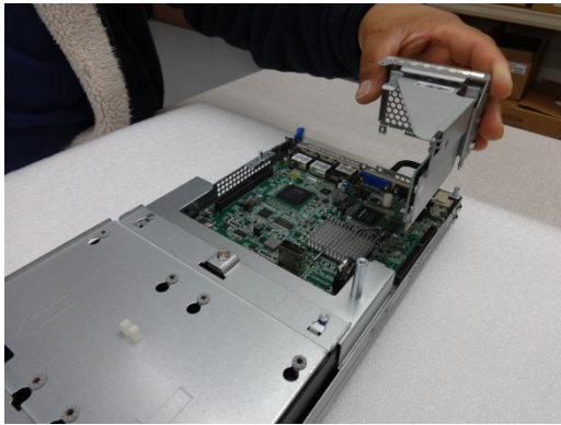
Unscrew Expander board bracket
