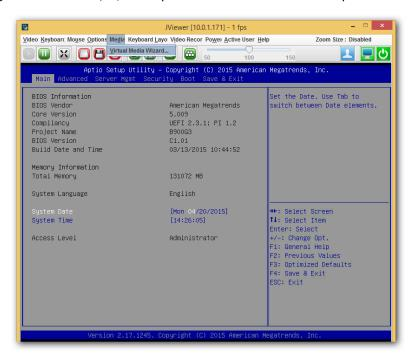
2. On this menu, you can mount your own media (i.e. Floppy Disk, CD/DVD, or HDD/USB) to the system. When finished, click 'Close'. The KVM/IP will require a Power Cycle if virtual media is mounted when system is on BIOS (screenshot below). If system is on OS, no reboot is needed as virtual media can be immediately accessed.
