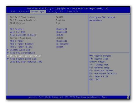
3. On 'BMC network configuration', the station IP address (i.e. 10.0.1.171) is your KVM/IP access to your system via web browser.
